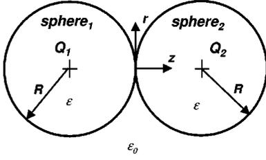
FIG. 1. Definition sketch of two touching dielectric spheres of equal size.
